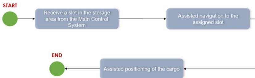
**Figure 3 Procedure Diagram — Transfer to Storage Area**
