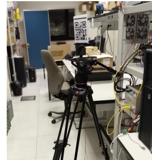
Servo- controlled QR code target used for calibration
